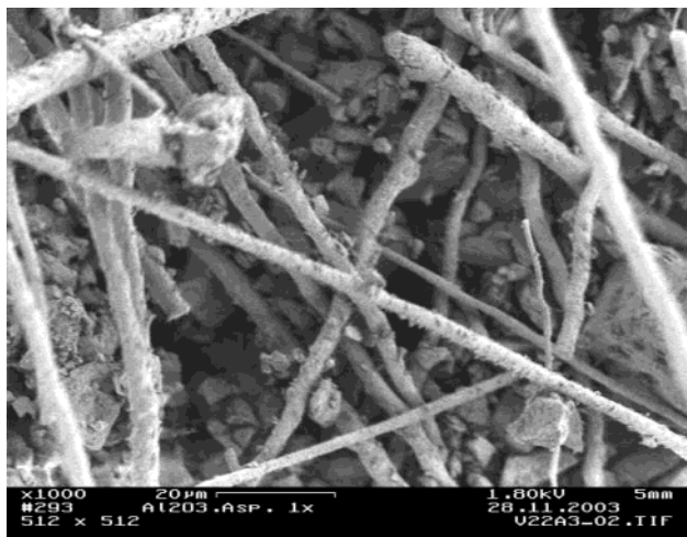
Figure 3. SEM micrograph of an AS-R biocer body.
